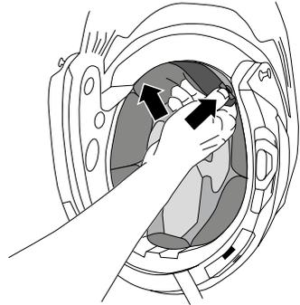
2. Insert the plastic retention flaps with round holes over the pins sewn into the rear section of the cheek pad and affix them using the red snaps.
