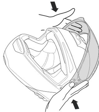
2. The face shield will then audibly lock into place when you press it gently towards the helmet with a simultaneous closing movement.
